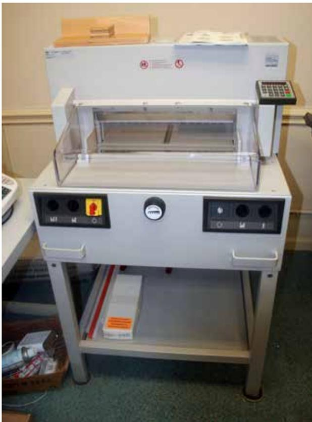
**Triumph 4850-95EP** programmable 18.5' x 19' behind knife paper cutter, 3" cutting height, 13.60" in front of knife, two blades with machine, electrical 115 V AC, 20 amp dedicated breaker, purchase new for over 8,000 and is in "like new" condition.
