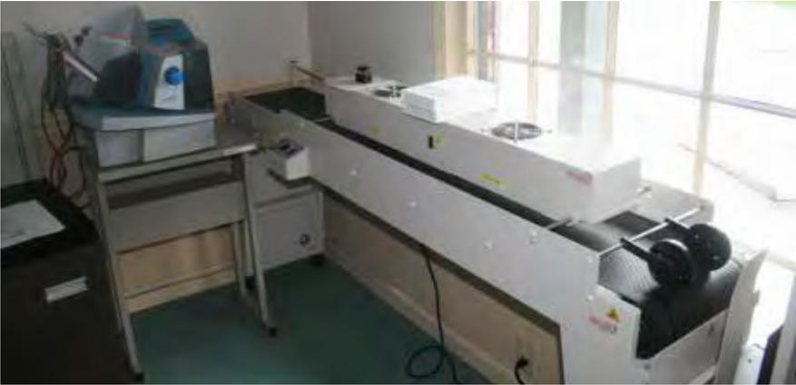
**Seacap SA 5000 Ink Jet Mailing Machine** with Seacap TCD 72 - 6' variable speed conveyor with two fan dryers on stand with castors for glossy and coated stocks. This equipment was purchased new and is "like new" condition. Specifications: Throughput (based on #10 envelopes) up to 22,000@hour; draft quality, 11,000@hour letter quality. Barcode, intelligent mail, USB or Ethernet; printhead/inkjet cartridge, media size 3" x 13"; 5" to 15.5" thickness up to 1/4".
