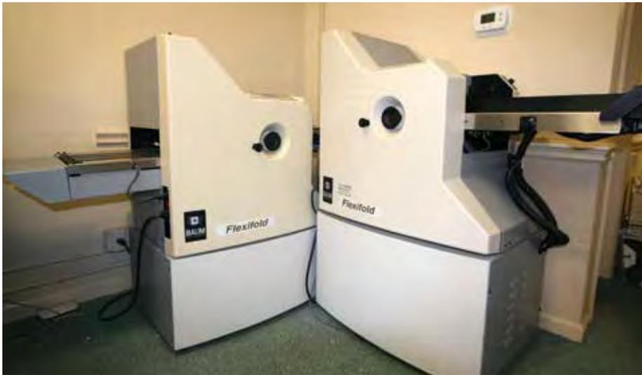
**Baum Flexifold** programmable vacuum fed right angle folder with large feed table and conveyor, perforation and scoring wheels. The specifications are as follows: Minimum sheet size, 3"x 5" to maximum sheet size of 14" x 20", minimum fold size is 2" with maximum paper weight of 65lb. cover. The fold roll speed is 1900@minute and 7200@minute. Electrical is 115 vac, 15 amp dedicated breaker. This machine was purchased new for over \$20,000 and is in "like new" condition.
